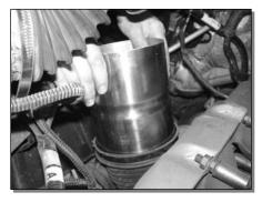
4. Install the **Flow Adapter** into the intake system using the clamps removed previously.
