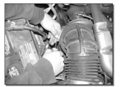
2. Remove the Clamps holding the intake tubes to the silencer. Do not discard the clamps as they are required for the installation of the **Flow Adapter**.
