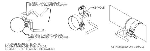
3. Install the **Muffler** onto the **Front Pipe** using the **Hang Tight<sup>TM</sup> Hanger Clamp Assembly**. Then install the hanger into the factory rubber insulator. Do not tighten the **Clamp** at this time. **Refer to Figure 4**.
