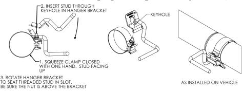
4. Slide the **Hang Tight<sup>TM</sup> Hanger** clamp assembly over the outlet of the **Extension Pipe**. Install the **Over-Axle Pipe** from the rear of the truck over the axle and slide on to the **Extension Pipe**. Install the **Hang Tight<sup>TM</sup> Hanger** into the factory rubber isolator.
