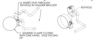
3. ROTATE HANGER BRACKET TO SEAT THREADED STUD IN SLOT. BE SURE THE NUT IS ABOVE THE BRACKET
