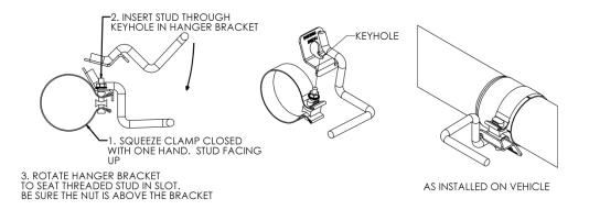
3. Slide the **Hang Tight<sup>TM</sup> Hanger Clamp** assembly onto the outlet end of the **4**" to **5**" Extension Pipe. Install the hangers into the existing OEM rubber insulators.
