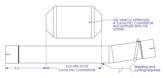
ADAPTOR PIPE TO WORK WITH 4" CATALYTIC CONVERTORS MAGNAFLOW 60011 (Federal compliance) or comparable product.
