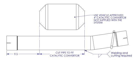
ADAPTOR PIPE TO WORK WITH 4" CATALYTIC CONVERTORS MAGNAFLOW 60011 (Federal compliance) or comparable product.
