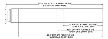
2. Mate the **Extension Pipe** flange to the stock exhaust flange with the **Gasket** between them and fasten the flanges together with the hardware provided.
