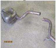
3. Cut the exhaust system right before the exhaust pipe goes over the rear subframe.
