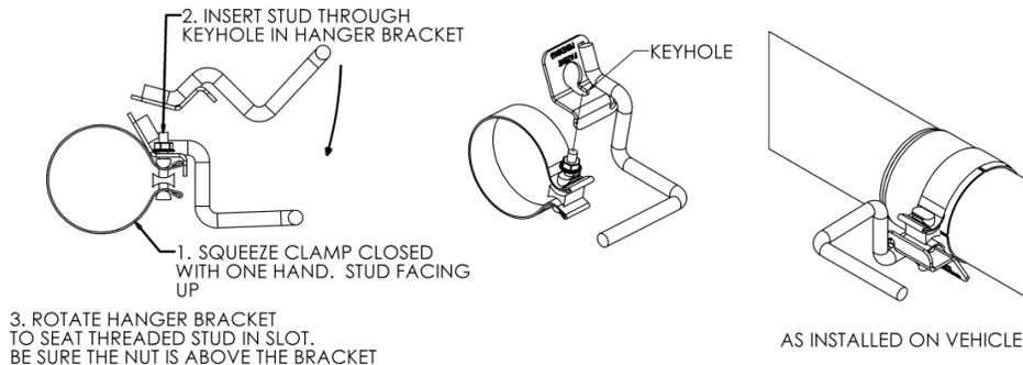
3. Install muffler onto extension pipe with the outlets horizontal. Loosely install the **Hang Tight™ Hanger Clamp Assembly** around the front muffler joint and into the factory rubber insulator located on the frame near the front of the muffler.
