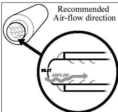
3. Install the **Muffler** over the required pipe so that the exhaust will flow smoothly over the louvers. Refer to the illustration on the left.
