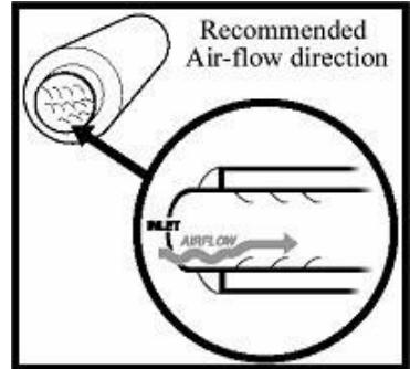
3. Install the **Muffler** over the **Extension Pipe** or over the **Mid Pipe** with 137" wheelbase vehicles. Refer to the figure on the left for correct **Muffler** orientation.
