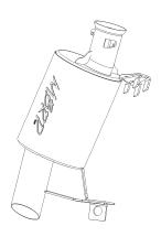
NOTE: To avoid exhaust leaks use high heat silicone to seal all connections between expansion chambers and muffler. Monitor for leaks during the first 200 miles after your installation and re-apply silicone where necessary. We suggest having your local snowmobile mechanic or performance shop install this product.
