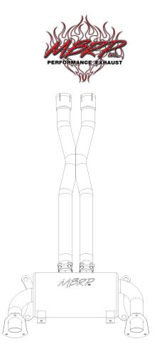
NOTE: To avoid exhaust leaks use high heat silicone to seal all connections between expansion chambers and muffler. Monitor for leaks during the first 200 miles after your installation and re-apply silicone where necessary. We suggest having your local snowmobile mechanic or performance shop install this product.
