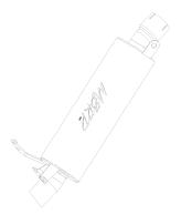
NOTE: To avoid exhaust leaks use high heat silicone to seal all connections between expansion chambers and muffler. Monitor for leaks during the first 200 miles after your installation and re-apply silicone where necessary. We suggest having your local snowmobile mechanic or performance shop install this product.
