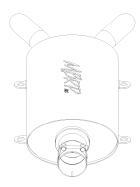
NOTE: To avoid exhaust leaks use high heat silicone to seal all connections between expansion chambers and muffler. Monitor for leaks during the first 200 miles after your installation and reapply silicone where necessary. We suggest having your local snowmobile mechanic or performance shop install this product.
