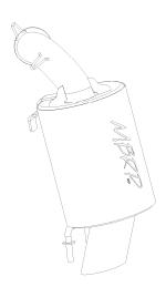
NOTE: To avoid exhaust leaks use high heat silicone to seal all connections between expansion chambers and muffler. Monitor for leaks during the first 200 miles after your installation and re-apply silicone where necessary. We suggest having your local snowmobile mechanic or performance shop install this product.
